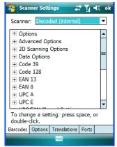
The dropdown menu to the right of the *Scanner* option allows you to choose from one of the following scanner types used with your Ikôn: *Decoded (internal)*, *Decoded (Internec ISCP)* or *Imager*.
